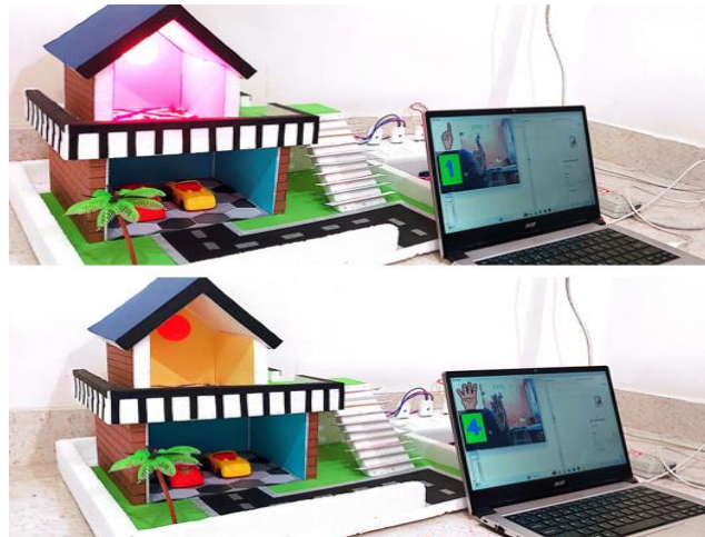
Figure 5: 1 st Hand Gesture- Light 1 ON, 4 th Hand Gesture- Light 1 OFF
