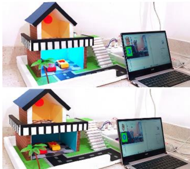
Figure 7: 3 rd Hand Gesture- Light 3 ON, 0 th Hand Gesture- Light 3 OFF
