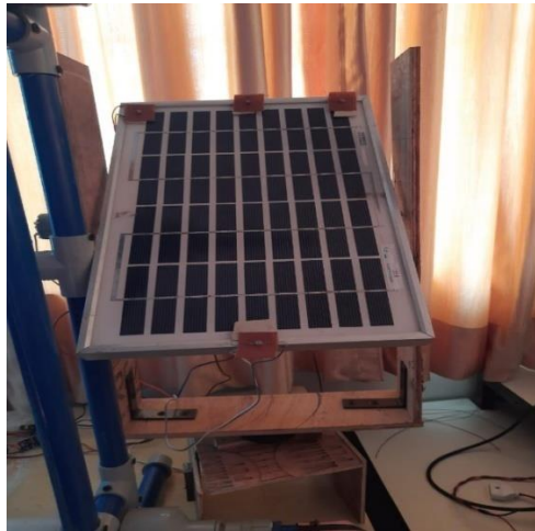
Figure 7. The dual axis solar panel (front view)
