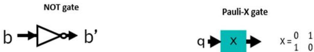
Figure 1. Comparison of Classical NOT gate in Boolean Algebra and equivalently performing Pauli-X gate.
