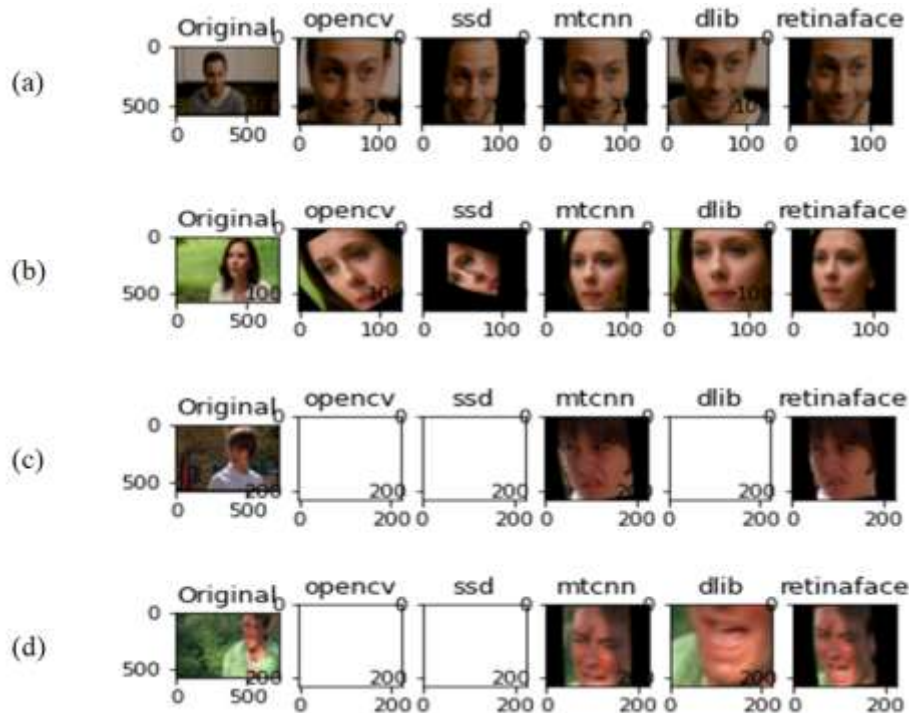
Figure 3. Face detection using the Deepface framework. (a)Frontal face detected by all detectors. (b) The Face is detected by all but not properly aligned by OpenCV and SSD. (c) Variation in a head pose is only detected by MTCNN, Retinaface. (d) MTCNN, Retinaface detectors are only successful on Head pose variation and illumination effects.
