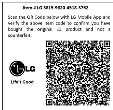
Fig. 2 QR Code encoding an encrypted LG product item code
